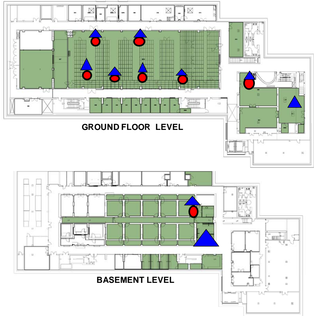
Figure 1: Locations of safety showers and eye washes.
